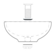
4. Apply a bead of silicone slightly form the edge of the basin.
